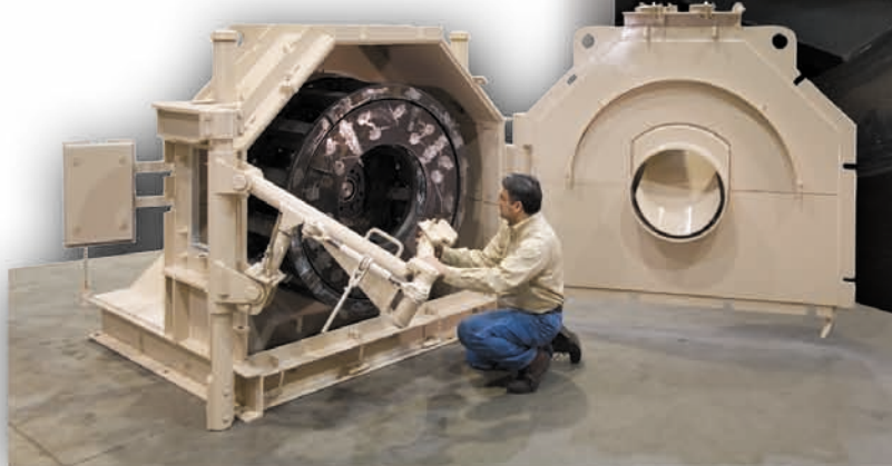
This Model 50B-2C4R CAGE-PAKTOR with an optional jib crane is ready to remove cages.
